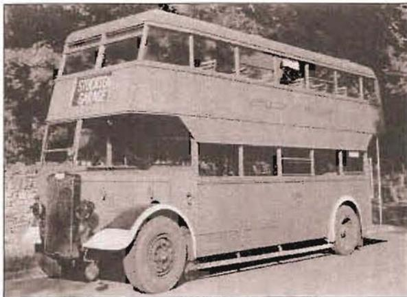
A typical utility double decker. This is 6LW powered Arab Mk.II chassis with a lowbridge body built in Leeds by Charles H Roe
